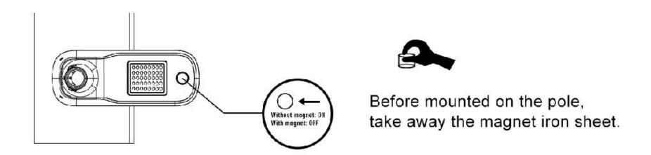
The internal battery is locked from factory for safety shipment, so users have to take away the magnet iron sheet to unlock the battery and lighting system.
